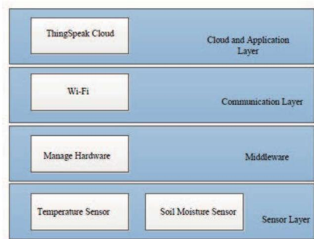
Fig. 1. Different layers of smart Farming System
