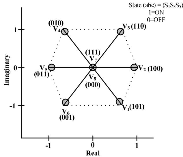
Fig. 3: Voltage vectors of a 2level 3ph inverter
