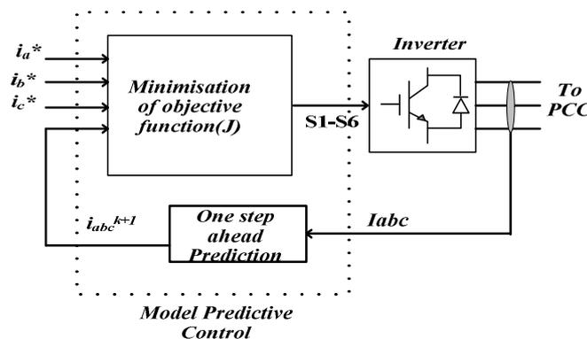
Fig. 2: Model Predictive Control based Current Control of Three phase inverter
