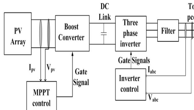
Fig. 1: Two stage Grid connected PV system
