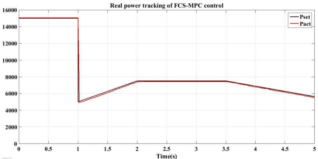
Fig. 4: Real power set point tracking performance of FCS-MPC control based on ISCT
