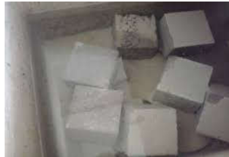
CURING OF CUBES
