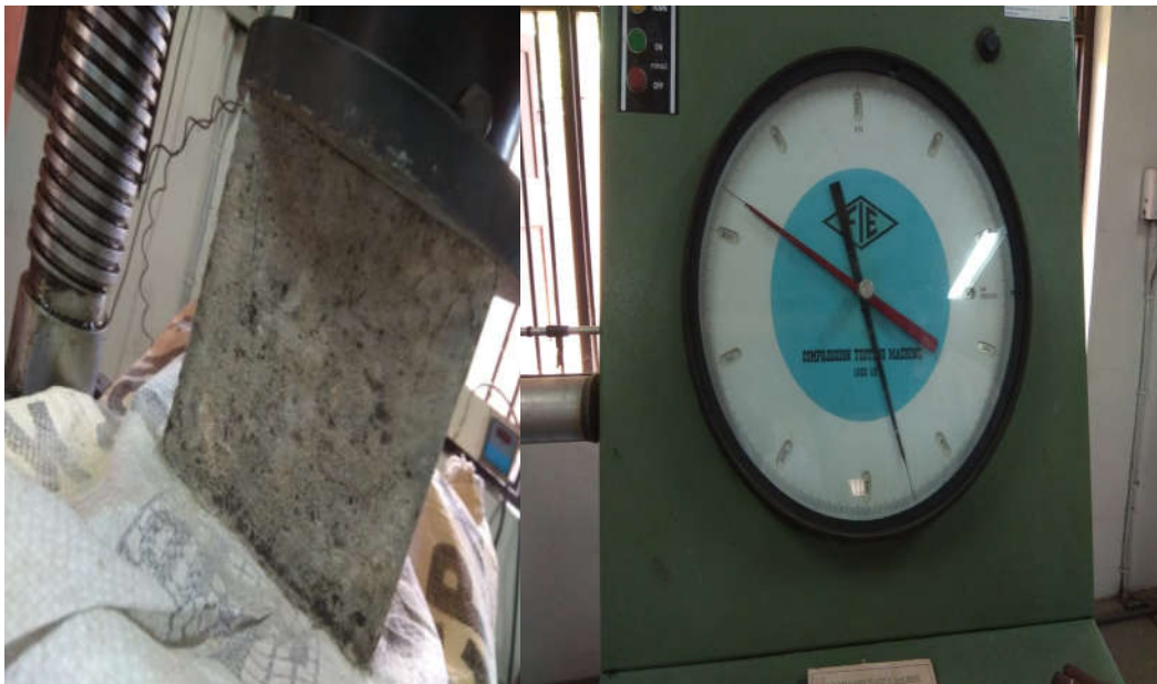
Fig 4. Compressive strength of cubes
