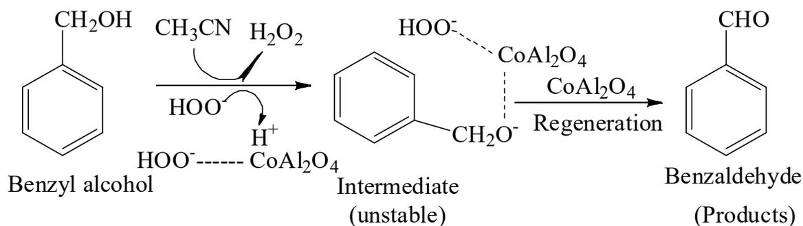
**Figure 4.2.11.** Schematic diagram of catalytic oxidation of benzyl alcohol into benzaldehyde by spinel  $\text{CoAl}_2\text{O}_4$  catalyst.
