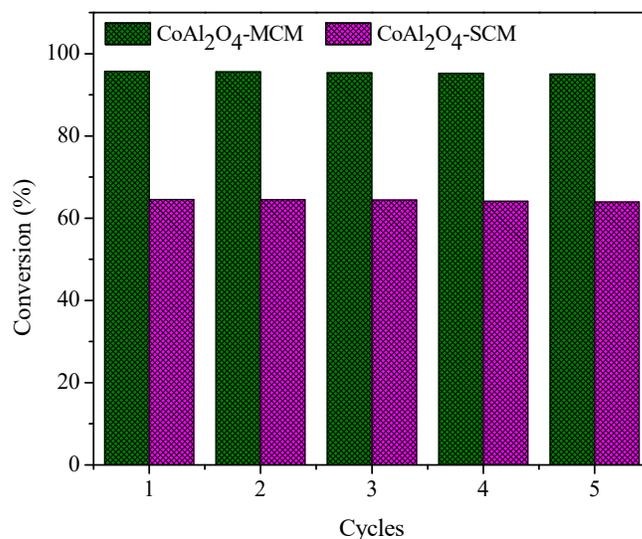
**Figure 4.2.12.** The reusability of the spinel catalysts (CoAl<sub>2</sub>O<sub>4</sub>-MCM and CoAl<sub>2</sub>O<sub>4</sub>-SCM) for the catalytic oxidation of benzyl alcohol into benzaldehyde.
