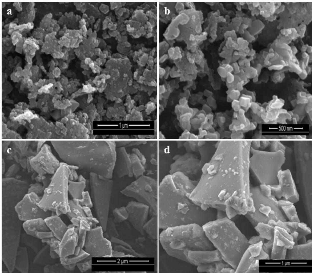
**Figure 4.2.3.** HR-SEM of  $\text{CoAl}_2\text{O}_4$ : (a, b)  $\text{CoAl}_2\text{O}_4$ -MCM and (c, d)  $\text{CoAl}_2\text{O}_4$ -SCM
