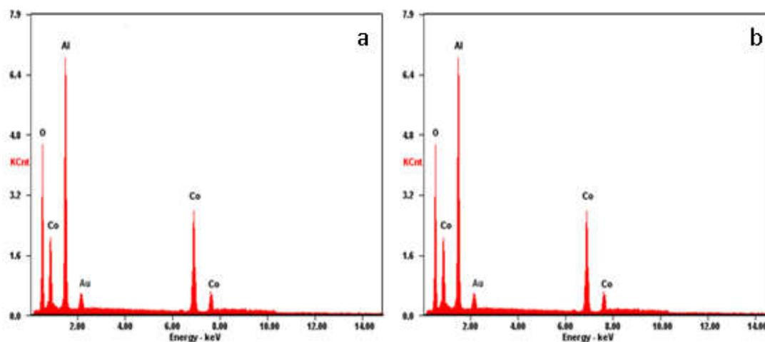
**Figure 4.2.5.** EDX spectrum of  $\text{CoAl}_2\text{O}_4$ : (a)  $\text{CoAl}_2\text{O}_4\text{-MCM}$  (b)  $\text{CoAl}_2\text{O}_4\text{-SCM}$
