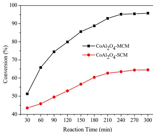
**Figure 4.2.10.** The catalytic reaction time of CoAl<sub>2</sub>O<sub>4</sub>-MCM and CoAl<sub>2</sub>O<sub>4</sub>-SCM samples on the conversion towards the oxidation of benzyl alcohol into benzaldehyde (Reaction conditions: Catalyst (0.1g to 0.8 g); Benzyl alcohol, 5 mmol; Acetonitrile, 5 mmol; H<sub>2</sub>O<sub>2</sub>, 5 mmol; Temperature, 80 °C, time, 5 h).
