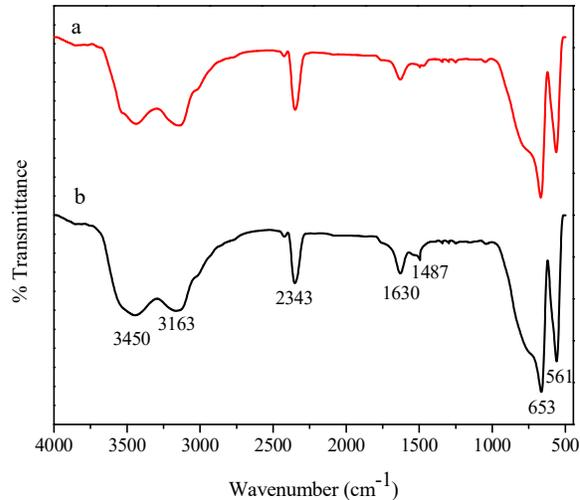
**Figure 4.2.2.** FT-IR spectra of  $\text{CoAl}_2\text{O}_4$ : (a)  $\text{CoAl}_2\text{O}_4$ -MCM (b)  $\text{CoAl}_2\text{O}_4$ -SCM
