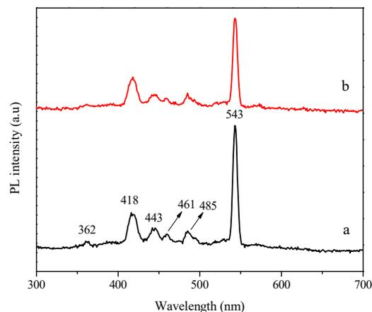
**Figure 4.2.7.** Room temperature PL spectra of  $\text{CoAl}_2\text{O}_4$ : (a)  $\text{CoAl}_2\text{O}_4$ -MCM (b)  $\text{CoAl}_2\text{O}_4$ -SCM.
