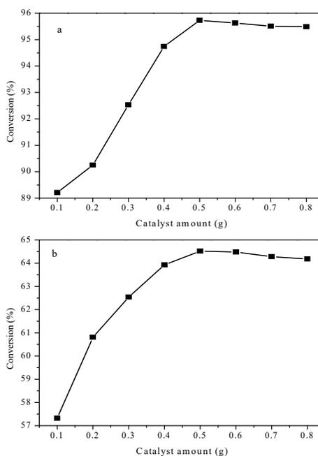
**Figure 4.2.9.** The amount of spinel catalysts of  $\text{CoAl}_2\text{O}_4$ -MCM (Fig. 9a) and  $\text{CoAl}_2\text{O}_4$ -SCM (Fig. 4.2.9b) samples on the conversion towards the oxidation of benzyl alcohol into benzaldehyde (Reaction conditions: Catalyst (0.1g to 0.8 g); Benzyl alcohol, 5mmol; Acetonitrile, 5mmol;  $\text{H}_2\text{O}_2$ , 5mmol; Temperature,  $80^\circ\text{C}$ , time, 5h).
