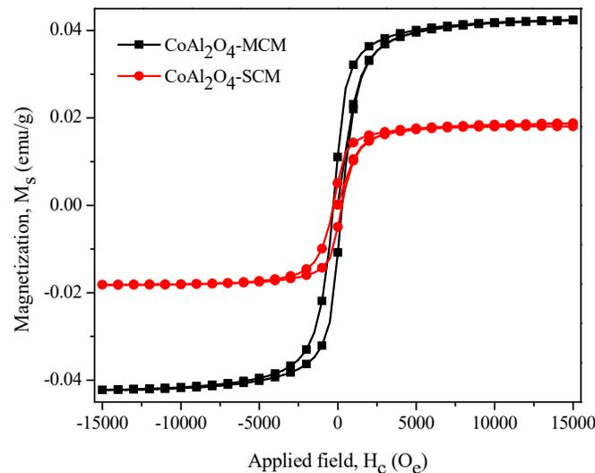
**Figure 4.2.8.** Magnetic hysteresis (M-H) loop of  $\text{CoAl}_2\text{O}_4$ -MCM and  $\text{CoAl}_2\text{O}_4$ -SCM samples
