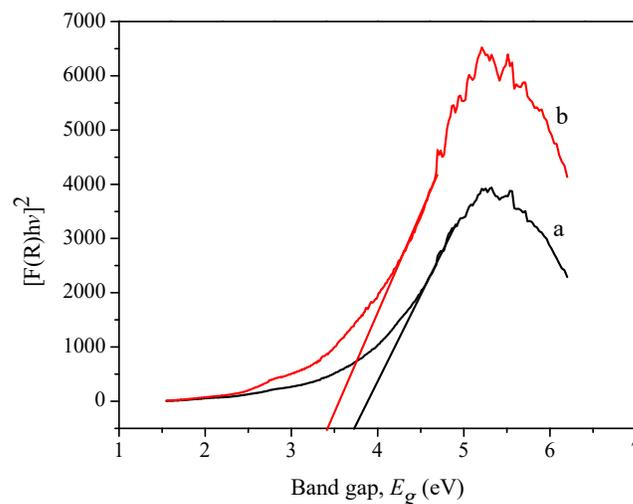
**Figure 4.2.6.** UV-Visible diffuse reflectance spectra (DRS) of  $\text{CoAl}_2\text{O}_4$ : (a)  $\text{CoAl}_2\text{O}_4\text{-MCM}$  (b)  $\text{CoAl}_2\text{O}_4\text{-SCM}$
