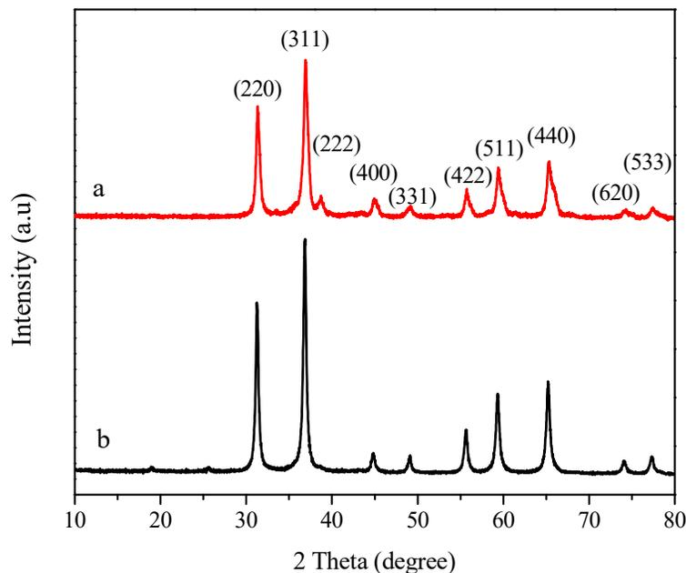
**Figure 4.2.1.** XRD pattern of  $\text{CoAl}_2\text{O}_4$ : (a)  $\text{CoAl}_2\text{O}_4$ -MCM (b)  $\text{CoAl}_2\text{O}_4$ -SCM
