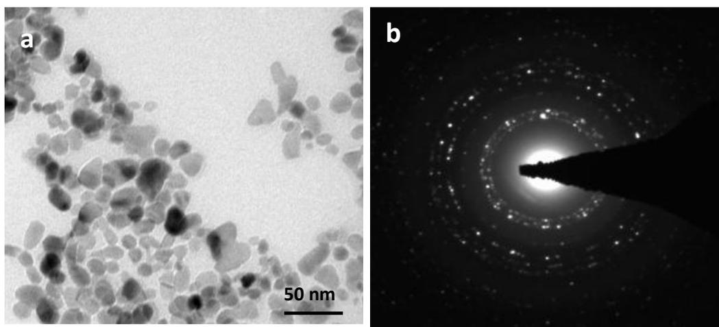
**Figure 4.2.4.** HR-TEM image (a) and SAED pattern (b) of  $\text{CoAl}_2\text{O}_4$ -MCM
