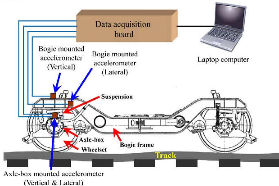
**Figure 1. Block diagram of ABA**
