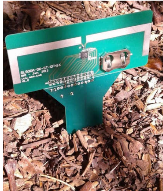
Figure 8. Example of the Soil Stick Sensor for Humidity in a real situation.
