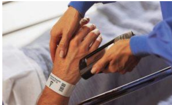
Fig.1 – NFC Device and hand tag
