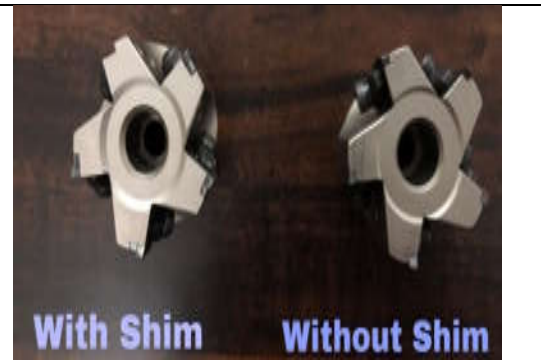
Fig. 1.(b) face milling tool 63 mm dia with shim and Without shim face mill
