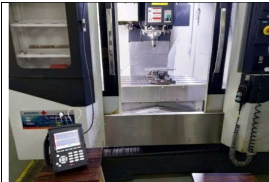
Fig. 1.(a) CVM milling Machine with CoCo80 Dynamic Signal analyser with Try Axial Sensor
