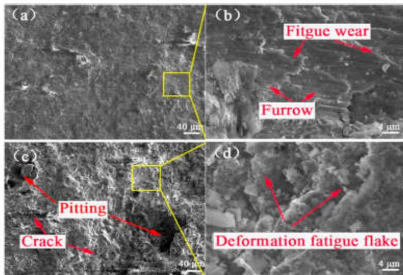
Fig. 9 – Observation of worn surface of BDI B after impact wear under (a, b) 1J and (c, d) 4J impact load.
