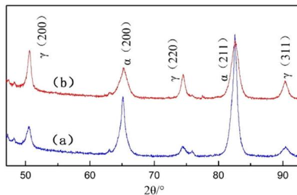
Fig. 3 – XRD curves of ductile irons for the BDI A (a) and BDI B (b).
