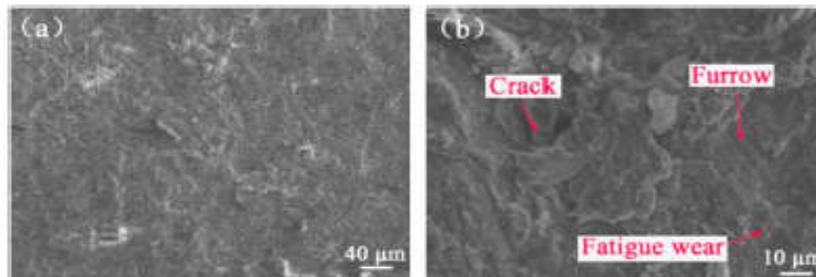
Fig. 8 – Observation of worn surface of BDI A after impact wear: (a) 1 J; (b) 4 J.
