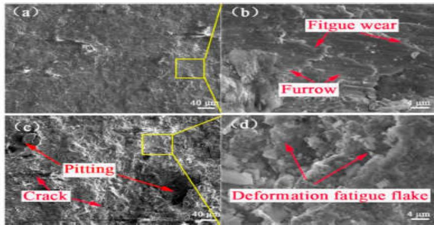
Fig. 9 – Observation of worn surface of BDI B after impact wear under (a, b) 1 J and (c, d) 4 J impact load.
