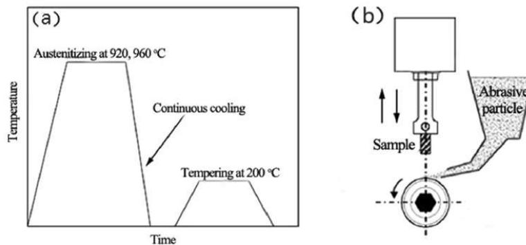
Fig. 1 – (a) Schematic diagram of continuous cooling process; (b) Schematic diagram of MLD-10 impact abrasive wear tester.
