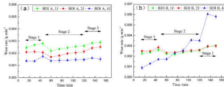
Fig. 5 – Wear rate variation of different samples with time: (a) BDI A; (b) BDI B.
