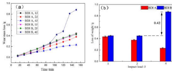
Fig. 4 – Wear mass loss with time (a) and total weight loss (b) of the samples under different load conditions.
