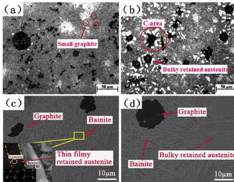
Fig. 2 – Microstructure at the initial state. OM image of (a) BDI A and (b) BDI B; SEM secondary electron (SE) image of (c) BDI A (the inset shows TEM micrograph and selected area diffraction pattern (SADP) of austenite and bainite and the white circles indicate areas from where SADP were taken) and (d) BDI B.
