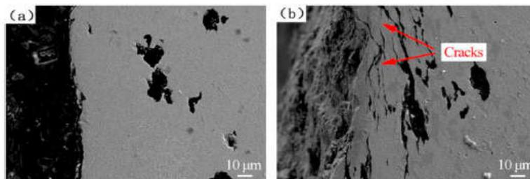
Fig. 7 – The cross section of samples after impact wear test under 4 J: (a) BDI A; (b) BDI B.
