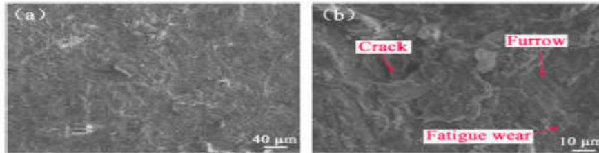
Fig. 8 – Observation of worn surface of BDI A after impact wear: (a) 1 J; (b) 4 J.
