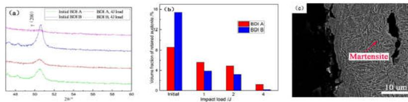
Fig. 6 – XRD curves for samples before and after wear test (a); volume fraction of retained austenite of different samples (b); microstructure of BDI B after wear test at 4 J (c).
